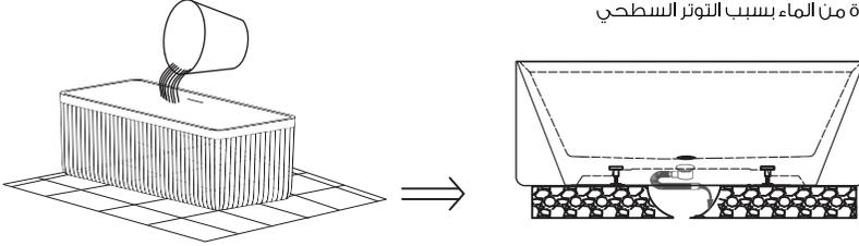
Finally you need to do a final test for drainage.
