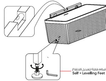
Adjust the self-levelling feet such that the Bath is level.
